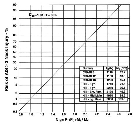
FIGURE 5.7. Risk of AIS  $\geq$ 3 neck injury as a function of combined normalized neck extension moment taken with respect to the occipital condyles and neck
