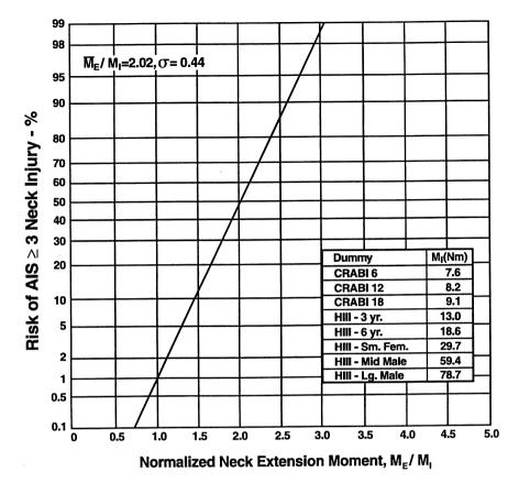
FIGURE 5.5. Risk of AIS  $\geq$ 3 neck injury as a function of normalized neck extension moment for the CRABI and Hybrid III dummy families. Minimum muscle tone.
