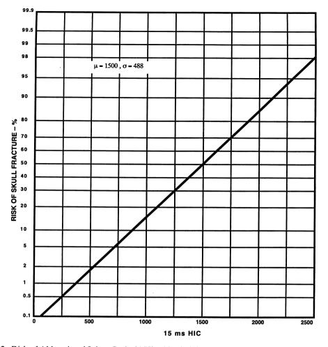
FIGURE 5.2. Risk of Abbreviated Injury Scale (AIS)  $\geq$ 4 brain injury as a function of 15-ms HIC for forehead impacts.
