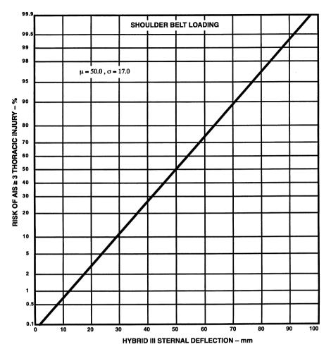
FIGURE 5.9. Risk of AIS  $\geq$ 3 thoracic injury due to shoulder belt loading of the thorax as a function of sternal deflection for the Hybrid III midsize male dummy.
